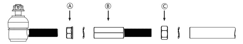
※ Safety adjustment length: 40mm 調整安全長度40mm
