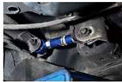
#6111-S REAR TOE ARM Toe arms allow for fine-tuned adjustments to the rear toe in/out setting of the vehicle. It helps to raise straight line stability and road control. Pillow ball bushing equipped.
