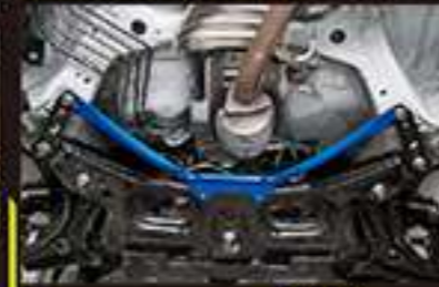
FRONT MIDDLE BRACE Behind the front sub-frame
