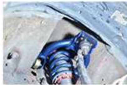
#6205 FRONT UPPER CAMBER KIT Pillow Ball Bushing Equipped with a camber adjustment function. Provide advanced stability and accurate response steering, especially during high speed driving and cornering.
