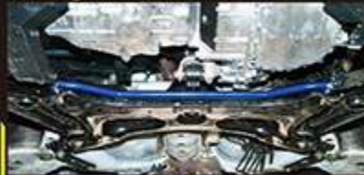
FRONT LOWER BRACE Connecting between control arm
