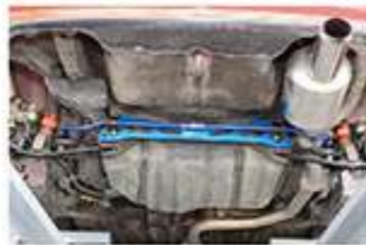
#8856 REAR SWAY BAR & SUB-FRAME BRACE Hardrace sway bars are designed to reduce body roll, and improve handling during performance-driving. Our sway bars are stiffer, more resilient and durable than factory sway bars. Compound with rear sub-frame brace are designed to stiffen up the chassis and reduce vehicle chassis flex. This will increase the rigidity of your car during high speed driving and hard cornering.
