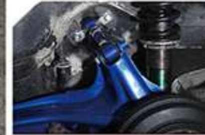
#7767 LIGHTWEIGHT TUBULAR FRONT LOWER CONTROL ARM Lightweight design, weight saving of 2.1kg/4.5lbs per side, total unsprung weight saving of 4.2kg/9lbs. Pillow Ball Bushing Equipped. Dramatically improving handling performance.
