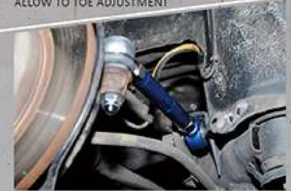
# 6392 REAR TOE CONTROL ARM ALLOW TO TOE ADJUSTMENT
