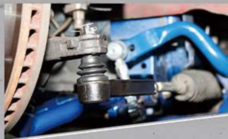
# 7699 RC TIE ROD END CORRECT LOWERED GEOMETRY
