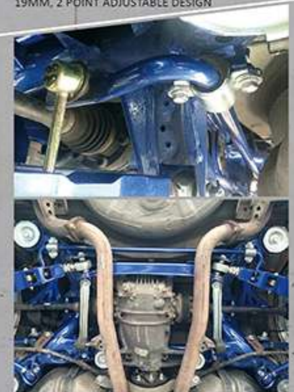
# 7746 REAR SWAY BAR 19MM, 2 POINT ADJUSTABLE DESIGN
