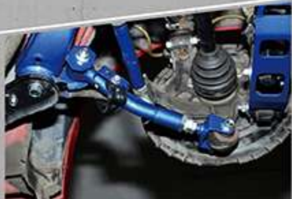
# 7593 REAR TRAILING ARM EXTREME SHORT FOR STANCE, ADJUST CASTER OF REAR WHEEL, 30 MM SHORTER THAN THE ORIGINAL PART
