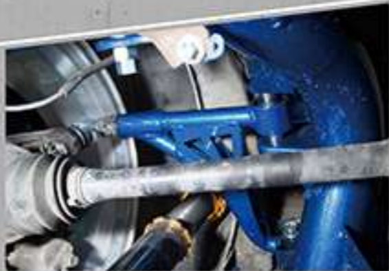
# 7540 REAR UPPER CAMBER KIT ALLOW TO CAMBER ADJUST
