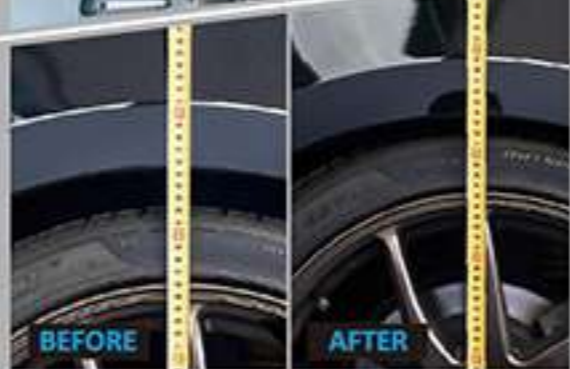
# 7401 REAR LOWER ARM EXTREME LOW USE, FOR CAR LOWER 20MM AND 40MM
