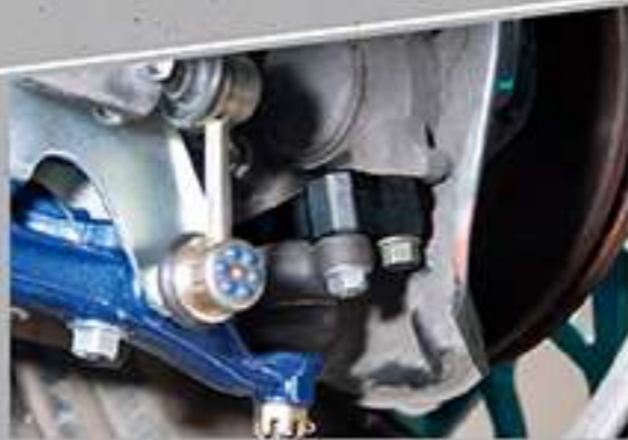
# 7859 ROLL CENTER ADJUSTER 30MM INCREASE + NEGATIVE CAMBER - 6 DEGREE
