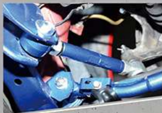
# 6753 REAR TOE ARM ALLOW FOR FINE-TUNED ADJUSTMENTS TO THE REAR TOE IN / OUT SETTING
