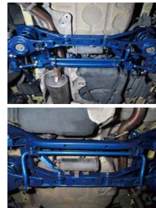
#7656-300 FRONT ADJUSTABLE STAB. LINK Range: 280-319mm
