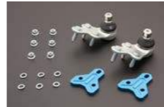
#7652 RC BALL JOINT 10mm HEIGHT ADDED
