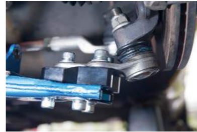
#7651 RC ADJUSTER ADD 20mm. CAMBER ADJUSTMENT
