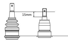
Length of ball stud is increased by 15mm to correct the horizontal position of front lower arm.
