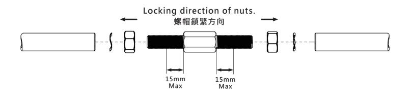
※ Safety adjustment length: Within 30mm 調整安全長度30mm以內
