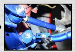
The camber kit allows fine adjustments to the rear end camber setting of the vehicle. It can either help maximize wheel contact patch to improve cornering grip or get your car back to original alignment specs after lowering to prevent uneven tyre wear. The arms are made of high tensile steel alloys to offer greatest strength and durability. The premium quality pillow ball bearings equipped also provide much more precise and solid handling response over the factory components.
