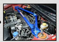
Rear Strut Brace are designed to reduce vehicle chassis flex. This will increase the rigidity of your car during high speed driving and hard cornering. This is why HARDRACE Rear Strut Brace can maximizes the performance and brings better handling feeling and quicker response.
