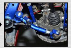
Toe arms allow for fine-tuned adjustments to the rear toe in/out setting of the vehicle. It helps to raise straight line stability and road control. Toe arm made with high-strength steel alloys to offer high durability, strength and yet remain light-weight.
