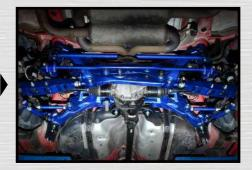
Fender Brace are designed to stiffen up the chassis and reduce vehicle chassis flex. This will increase the rigidity of your car during high speed driving and hard cornering.
