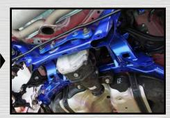
This will reduce vehicle chassis flex and deflection to increase the rigidity of your car under high speed driving and hard cornering, resulting in better and quicker handling response.
