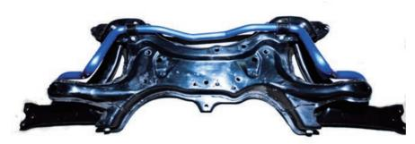
Removal of front sub-frame is suggested for easier installation.
