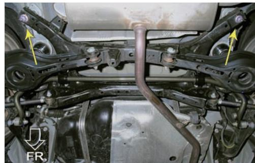
2. Install ①Brace to the vehicle using the removed bolts.
