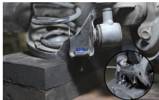
2. Assemble ③ and ④Lower bracket to both ends of ①Sway bar using supplied ⑤Flange nuts. (See components figure)
