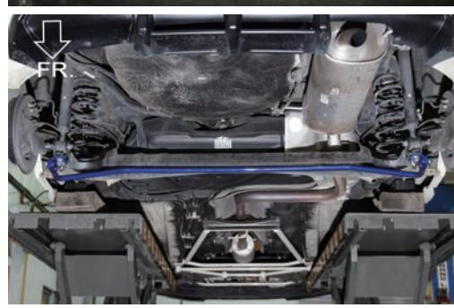
4. Once in place, install supplied ⑥Flange nuts with ⑦Spring washers and ⑧Washers to secure the sway bar. Then reinstall the shock absorbers to the axle beam. (See components figure & figure 2)
