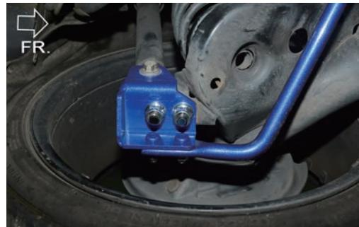
3. Position the sway bar to the axle beam by fitting the holes of the lower brackets to the upper bracket studs. (See figure 2)
