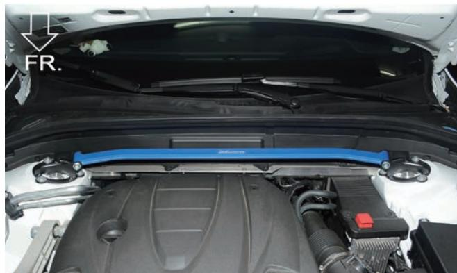
3. Install the cross bar to the brackets with supplied bolts, nuts and washers. (See components figure & figure 2)
