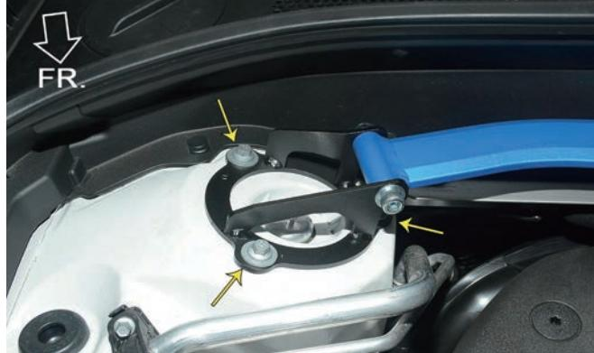
2. Position the brackets of ①Strut Brace to the strut towers on both sides, then reinstall the removed bolts to secure the brackets.
