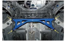
2. Once the brace is in place, reinstall the bolts to the subframe. 將拉桿固定後,沿用原螺絲將拉桿鎖上副車架。
