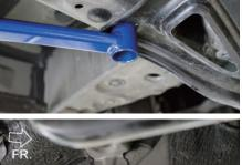
3. Position ① Mid-lower brace-RH and ② Mid-lower brace-LH as shown in the figures, then tighten using the original bolts.
