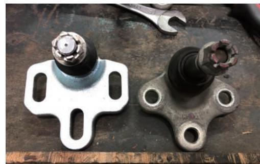
2. Install adjustable ball joints to the control arms. Adjust the ball joints to desired camber setting, then install supplied M12 bolts, nuts and washer plates to secure the ball joints.
