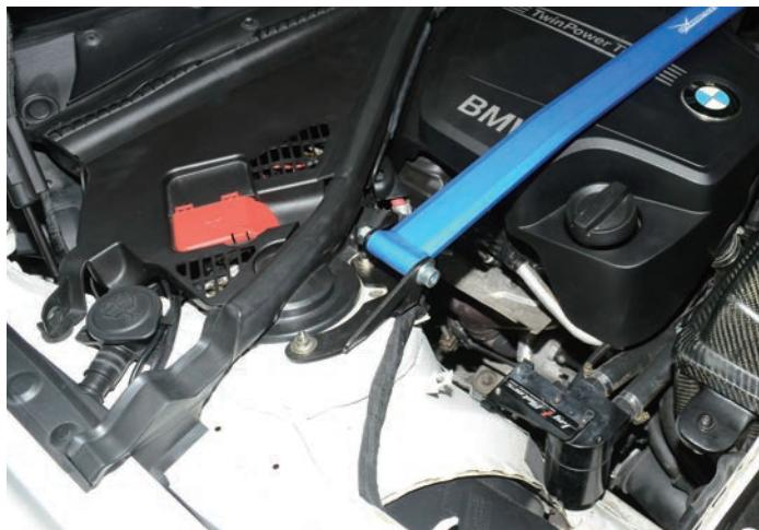
2. Position ① Strut brace over the mounts and tighten the nuts back.
