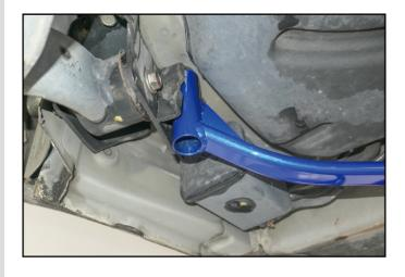
3. Reinstall the bolts to secure the brace. 鎖回螺絲以將桿身固定。
