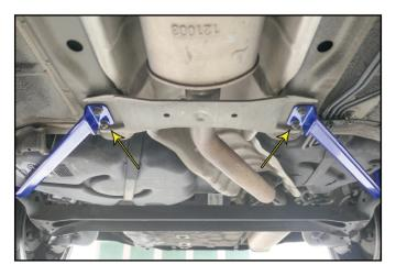
2. Position the brace on the vehicle. 安裝結構桿。
