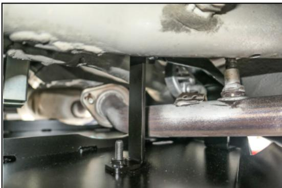
2. Install the washer with original nut. (do not screw all the way in, left about 3-5 threads at the top of the nut.)
