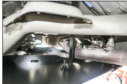
5. Last step is make sure screw all the nut all the way in. Make sure the plate is stable.
