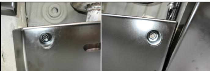
4. Using the M8x1.25x30 Bolt screw through the plant and C-clamp bracket.
