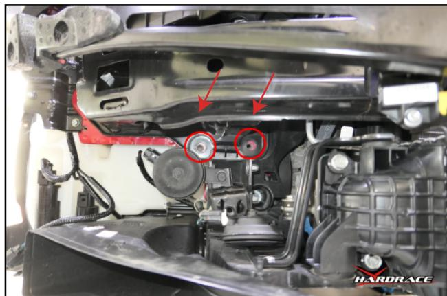
3. If you want to keep the honeycomb bumper. You need to cut a hole at the front of the hook adapter.
