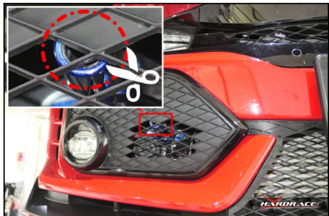
2. Using M10x1.25x40 bolt screw on the hook adapter.
