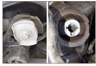
3. Reinstall the metal plate to the subframe bushings.
