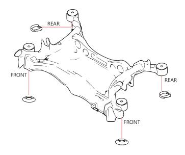
$\,$  2. Place the inserts into the voids of subframe bushings.
