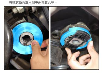
1. Remove factory metal plate and rubber retainer from the rear subframe bushings.
