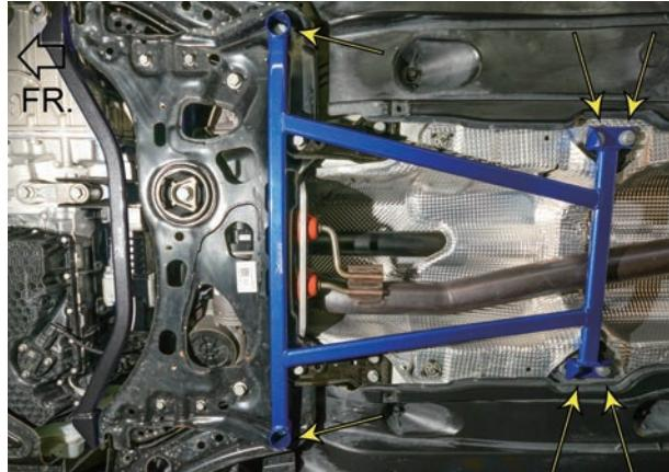
2. Install Brace to the vehicle. Then reinstall the bolts to secure the brace.
