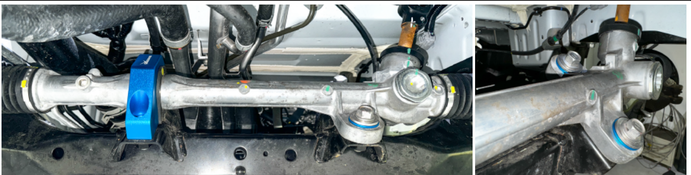
Illustration of installed state 安裝完成示意圖
